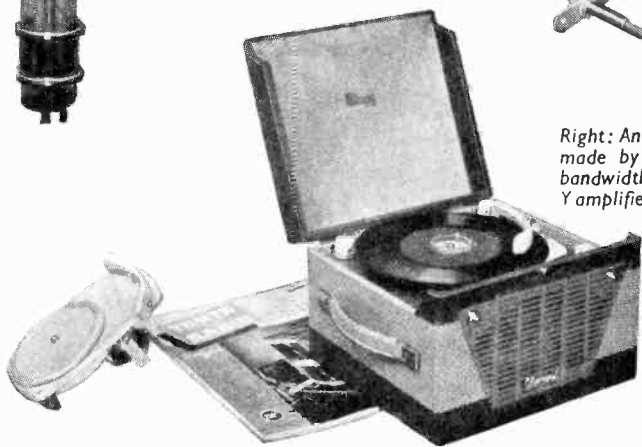
Left: A miniature gramophone turntable (45 r.p.m.) made by Eden-Dentzer. Right: The same equipment in a small portable record player by Clement, using a transistor amplifier (OC70, OC71 and two OC72s) and powered by four 1.5-V torch batteries. The size of the exhibits can be seen from the copy of our French contemporary, Toute La Radio , underneath.
