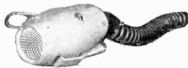
Left: Microphone incorporating a transistor pre-amplifier, shown by Lemonne.
