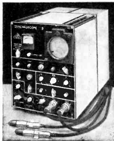
Right: An oscilloscope made by Leres. The bandwidth of the Y amplifier is 60 Mc. s.
